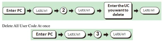
Remark : Auto-locking and Keypad locking function will be invalid when User Codes are deleted. The lock can only be operated by key during the time.
