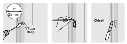
4. Install smart door sensor, then tighten the screws. For added security, install the smart door sensor and reinforcement plate.
