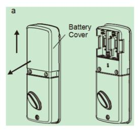
Insert 4 (AA) 1.5V alkaline batteries and put the battery cover back to the receiver module.
