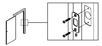
3. Locate center of strike hole by measuring back from door stop, 1/2 the thickness of door.
